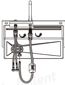
3. Install the cup cleaner and soap dispenser according to the line and tighten the nuts
