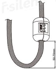
6. Install the drain according to the line and lock it tightly
