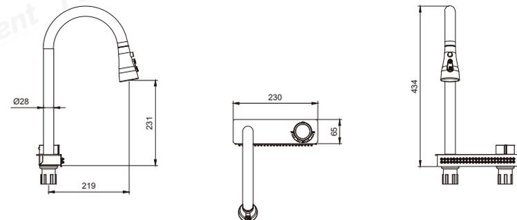
1. Put the faucet body onto the sink, make sure the hoses are in the correct holes.
